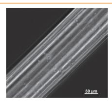
A photocrosslinkable microgrooved methacrylamide-modified gelatin (GelMA) fiber is produced via the use of a microfluidic device. The combination of the cell supportive properties of GelMA and the topographical cues allows improved cell-material interactions favoring anisotropic tissue formation. Moreover, the high hydration content and viscoelastic properties of the hydrogel allow the coculturing cell types in and on the fiber.
