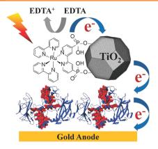
A molecular electron conduit of the decaheme cytochrome. MtrC. interfacing dye-sensitized TiO<sub>2</sub> nanocrystals to an electrode support is assembled and demonstrated. The constructed layers of MtrC and TiO<sub>2</sub> nanocrystals photosensitized with RuP are used in a biomimetic hybrid photobiochemical system with the aim to mimic the efficient spatial charge separation found in biological photosystems.
