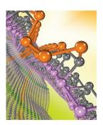
Phosphorene, a new member of the 2D materials, is in the spotlight. On page 2230 G. Zhang, Y.-W. Zhang and co-workers report a strong phononic anisotropy, unusual anharmonicity, and large structural flexibility in mono- and few-layer phosphorenes, which indicate that phosphorenes are promising for fabricating novel acoustic and thermal devices.
