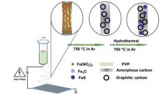
FeS nanodots accommodated in porous graphitic carbon nanowires are obtained via the combination of electrospinning technique and a biomolecular-assisted hydrothermal method. These materials exhibit excellent electrochemical performances as cathode materials. Key problems of conversion reaction, such as the low degree of reversibility and large polarization, are far-reachingly mitigated.
